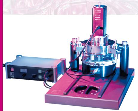
The innovative CULTEX® EDD is a modular designed electrical deposition device to increase the deposition efficiency for micro- and nanosized particles. In combination with the CULTEX® RFS or the CULTEX® RFS Compact, the CULTEX® EDD is applicable for a variety of cell culture inserts or even Petri dishes. The special design allows easy handling and cleaning and ensures reproducible results even with different aerosols and test substances.
