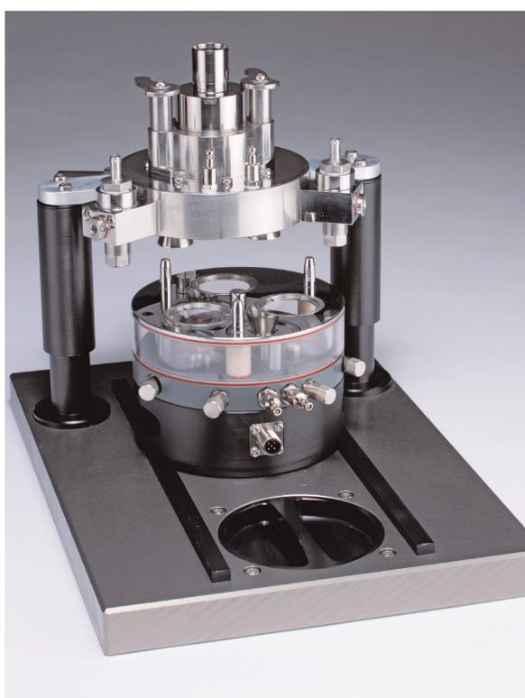
The CULTEX® Radial Flow System (RFS). Potential cytotoxic effects of the materials used were excluded by biomaterials testing prior to the construction.
