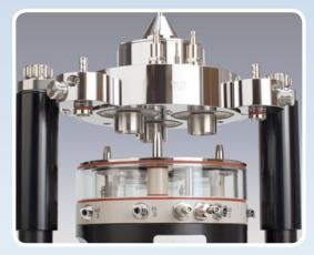
Here, the three individual gas inlets can be seen on the underside of the exposure top, fitting exactly into the insert vessels and thus realising a continuous flow of the test atmosphere above the test organisms regulated via flow controllers and a vacuum pump.
